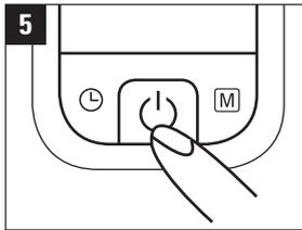
5 Start the measurement by pressing the Start/Stop button.
