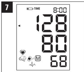
7 After the measurement the blood pressure values measured appear on the display.
