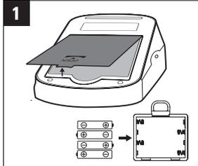
1 Insert the batteries supplied along with the monitor.
